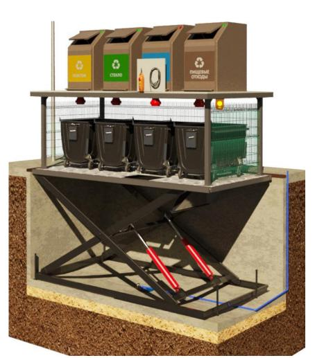
The ECOLIFT waste collection and underground storage system works on the principle of a hydraulic lift.
